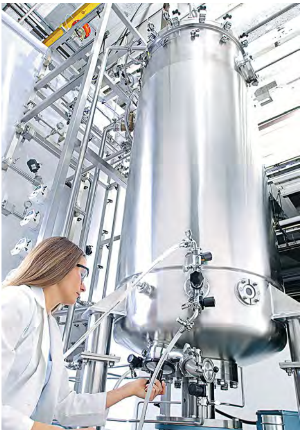
BioFlo Pro fermentors offer working volumes of up to 1,200 L.
