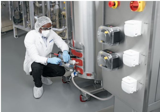
Easy to reach sensor location suitable for digital ISM and ARC sensors.
