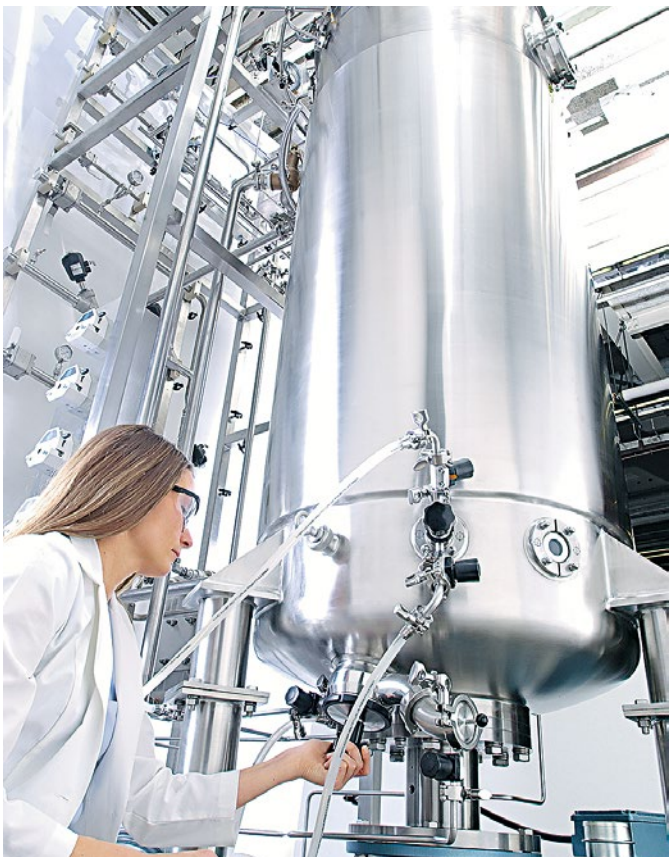
BioFlo Pro fermentors offer working volumes of up to 2,400 L.
