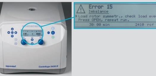
Eppendorf centrifuge families 58xx, 57xx, 5430/ R, and 5427 R have imbalance sensors to prevent spinning if the samples are not properly balanced. This protects device, sample, and user by preventing a rotor crash. Check with your provider for latest updates.
