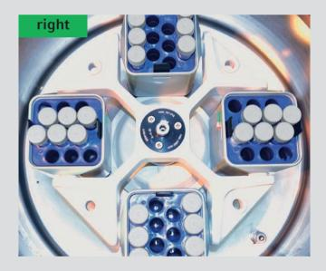
> Bucket and adapter loading must be symmetrical and balanced. > Position tubes in buckets in such a way that rotor pivots are stressed evenly. > Always have all 4 swing-buckets on rotor even though only 2 might be in use.
