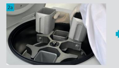
Remove buckets and rotor. For refrigerated centrifuges: > Defrost the ice on the rotor chamber surface. > Empty and clean the water collection tray.
