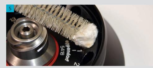
Wipe rotor chamber and motor shaft. If needed, wipe with mild neutral
