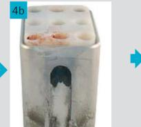
Check rotor and buckets for corrosion. Take out of service if corroded or if any sign of damage is detected.
