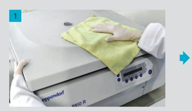
Switch off centrifuge and wipe centrifuge housing. If required, clean with mild detergents.
