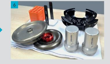
Place parts on dry cloth upside down to dry. To prevent aerosol-tight caps and seals from getting worn out/ damaged, store lids/caps separately from the bucket/rotor.
