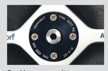
**Consider max. capacity** Note the weight specifications printed on the rotor (e.g.,  $4 \times 1.1$  kg means weights of each bucket + adapter + tubes filled with sample must not exceed 1.1 kg). Take note of the maximum g-force specified for the tubes you are using.
