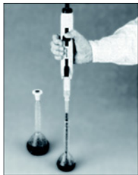
Fig. 4-6: Aspirating the liquid
