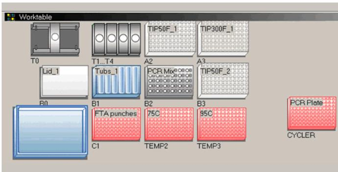
**Figure 1:** worktable set-up (Screenshot from the epMotion® Editor)
