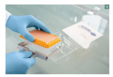
Optional: Remove tips or add tips from the reload rack (always work with full columns of tips).
