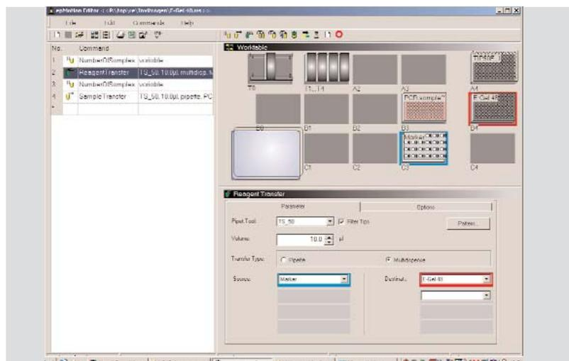
Fig. 2: epMotion Editor screenshot of the epMotion 5075 LH worktable with the labware for loading the E-Gel 48.
