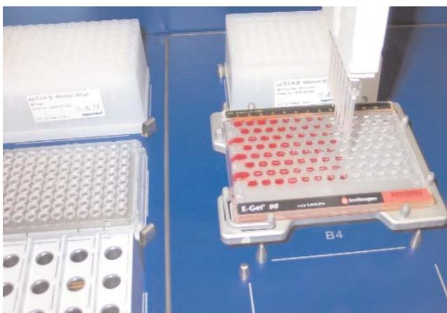
**Fig. 7:** Filling of the gel with the 8-channel dispensing tool
