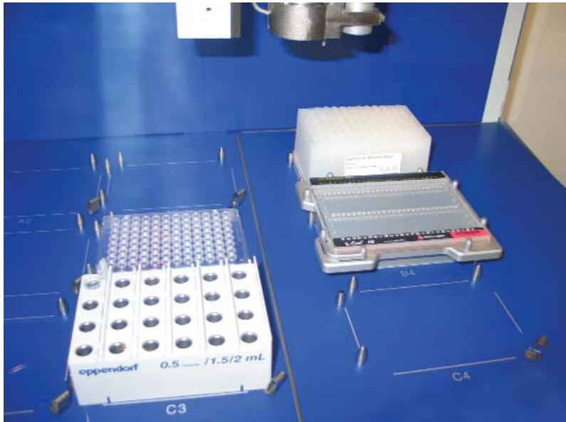
Fig. 1: The worktable of epMotion 5075 LH with the labware for loading of the E-Gel 48.
