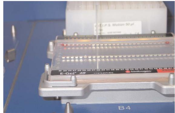
**Fig. 4:** Loading of the E-Gel 48 with the single-channel dispensing tool TS-50.
