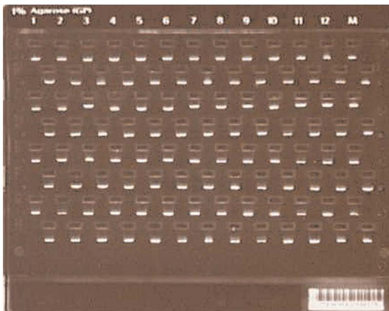
**Fig. 8:** 96 x 20  $\mu$ l plasmid DNA samples were loaded on a 1% Invitrogen E-Gel 96 with the epMotion 5075 LH. Electrophoresis was performed on the E-Gel Mother Base.
