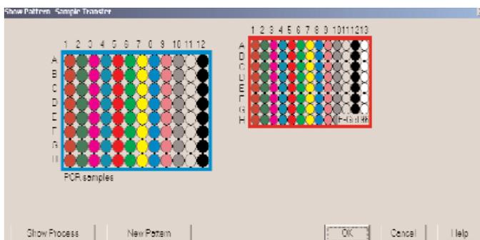
**Fig. 6:** The epMotion Editor screenshot: example of loading pattern for E-Gel 96. The 13th row remains free for the markers (pipetted by Reagent Transfer command with the single-channel tool TS-50).
