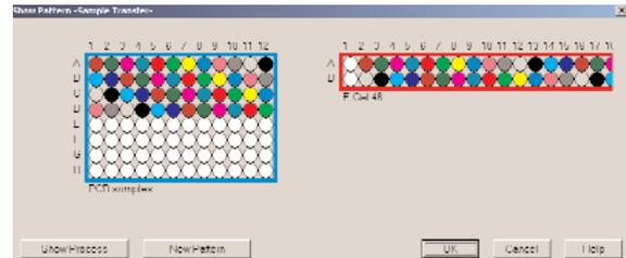
**Fig. 3:** The epMotion Editor screenshot version 9.22: example of loading pattern for E-Gel 48: 18 x 2 gel positions are visible. Please note: the epMotion control panel software makes 24 x 2 positions visible (not shown here).
