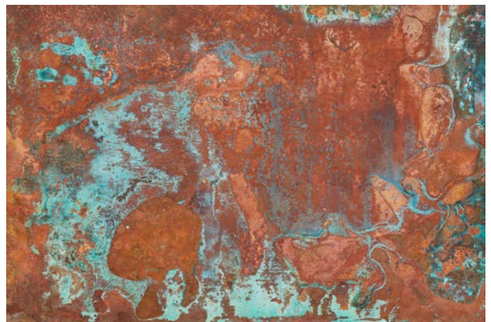
Fig. 2: An oxidized copper surface has stronger antimicrobial properties than a shiny copper surface
