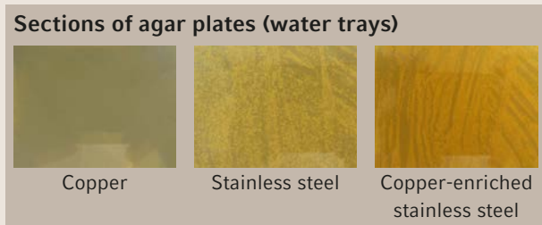
Fig. 4b: Results of the growth of S. cerevisiae on different surfaces in the CO 2 incubator (water trays: after 48 h incubation, shelves: after 24 h incubation)
