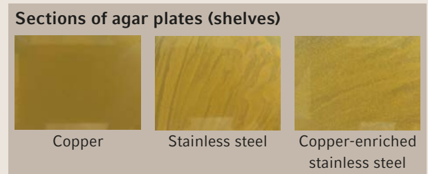
Fig. 4b: Results of the growth of S. cerevisiae on different surfaces in the CO 2 incubator (water trays: after 48 h incubation, shelves: after 24 h incubation)
