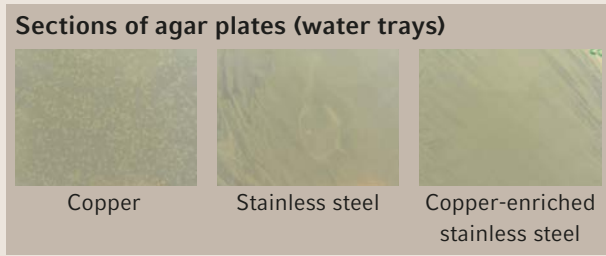
Fig. 4a: Results of the growth of E. coli on different surfaces in the CO 2 incubator
