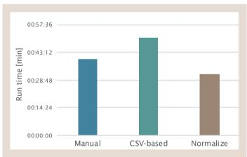
Processing time comparison for the normalization of 96 samples using water. Transfer from source 96 well plate to target 96 well plate. Diluent is presented in a reservoir.
