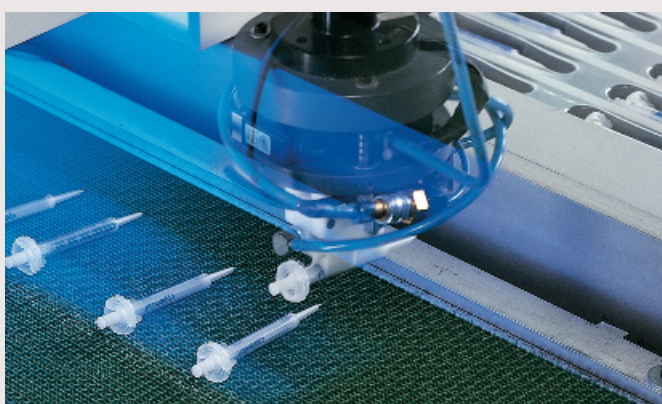
Fig. 2: Fully automatic sorting of Combitips into blister packs
