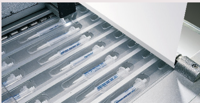
Fig. 3: Packing of consumables with Eppendorf purity grade Biopur prior to sterilization
