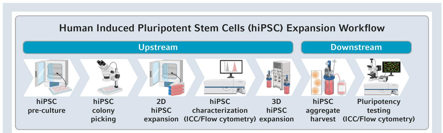
**Fig. 2:** hiPSC expansion workflow as aggregates in stirred-tank bioreactors (STB). Flow cytometry (FC) and immunocytochemistry (ICC) techniques were used to characterize hiPSC pluripotency. Created with BioRender.com.
