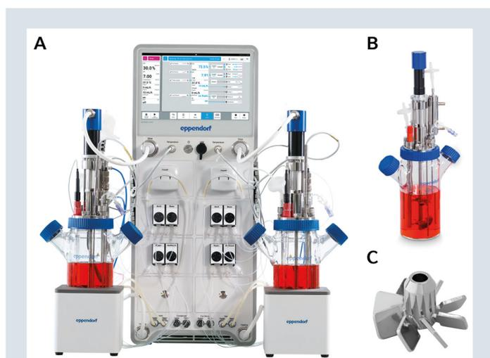
**Fig. 1:** (A) The SciVario twin bioreactor control system allows the control two single-use or glass bioreactors, either individually or in parallel, at the same time across a wide range of vessel sizes from small- to bench-scale. In this study, the (B) DASGIP Spinner vessel equipped with an (C) eight-blade pitched impeller specifically designed for the culture of shear-sensitive cells in suspension or as aggregates was employed.
