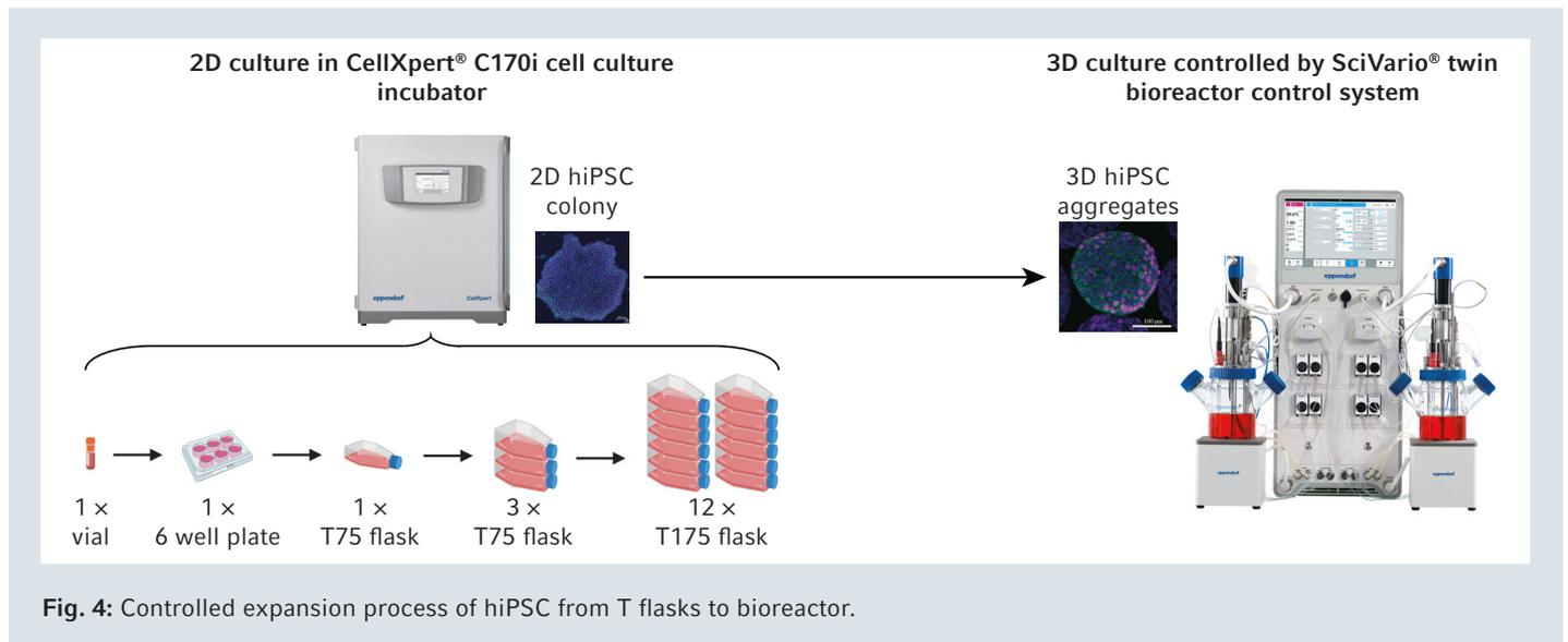
Fig. 4: Controlled expansion process of hiPSC from T flasks to bioreactor.
