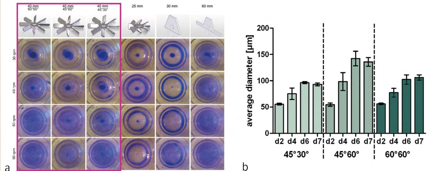
**Figure 1:** Impact of impeller design and stirring speed on mixing capabilities (left) and cell aggregate formation (right) in stirred suspensions using flat-bottom glass vessels (Ø 70 mm). **a** Stained microcarriers were stirred in 100 mL buffer for 10 min at different speeds. **b** Aggregate sizes of human induced pluripotent stem cells using three different pitched blade impellers were measured at day 2, 4, 6, and 7 of the culture in 2 – 3 independent runs each. [7]
