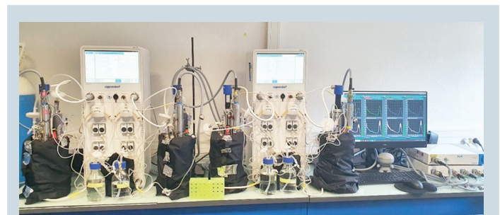
Fig 1A: SciVario twin – ProCellics Raman Analyzer Multi-Channel Unit setup in a dark environment used for the experiment shown in Figures 2 and 3 with opaque protections on the four bioreactors.
