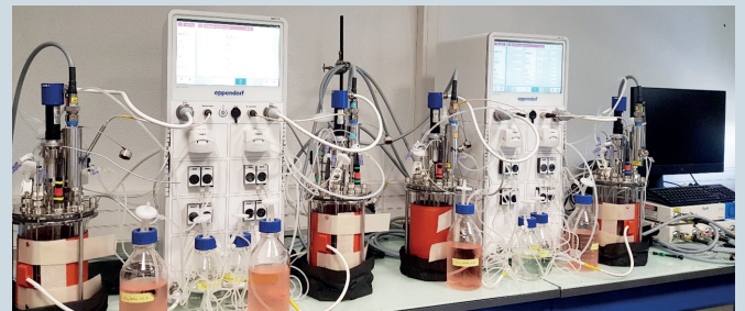
Fig 1B: SciVario twin – ProCellics Raman Analyzer Multi-Channel Unit setup in a light environment used for the experiment shown in Figure 5 without opaque protections on the four bioreactors.
