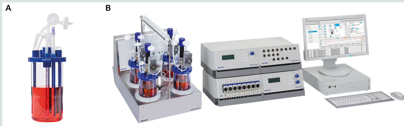
Figure 1: (A) BioBLU 1c Single-Use Bioreactors were used for k_La measurement in combination with the (B) DASGIP® Parallel Bioreactor System to control the relevant bioprocess parameters.
