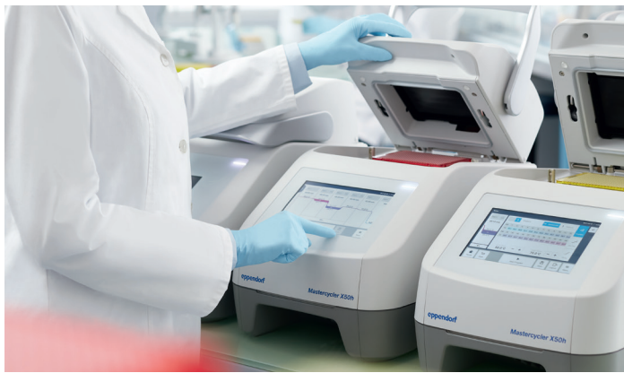
Figure 4: PCR cycler require energy due to constant heating and cooling steps
