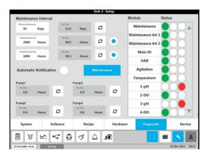
Monitoring the controller and the process is key to successful process development. The BioFlo 320 software features screens, designed to provide you with the status of both.
