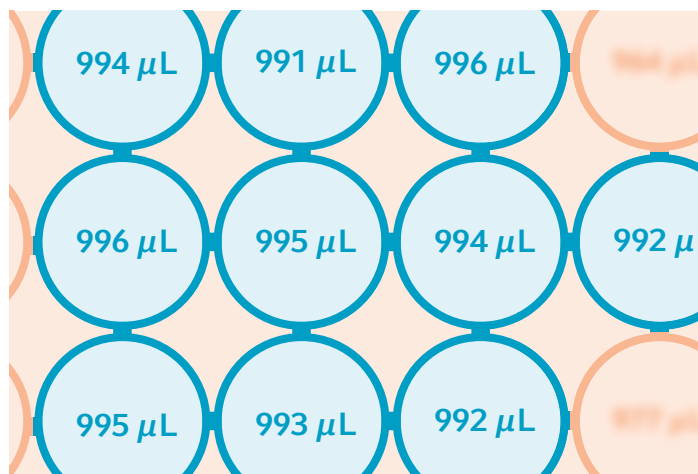
Ten measurements – average 993.77 \mu\text{L} , -0.62% systematic error
