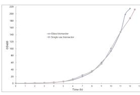
A high-cell density fedbatch cultivation of *E. coli* K12 in 3 L glass bioreactor and BioBLU 3f Single-Use Bioreactor, respectively, resulted in outstanding 200 OD<sub>600</sub> and highly similar growth curves—proving the excellent comparability of the bioreactor designs.
