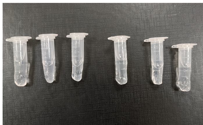
Figure 1: 1.5 mL microtubes with 20% recycling content from third-party supplier after centrifugation at 24,000x g and temperatures of up to +40°C, tubes are deformed during the run
