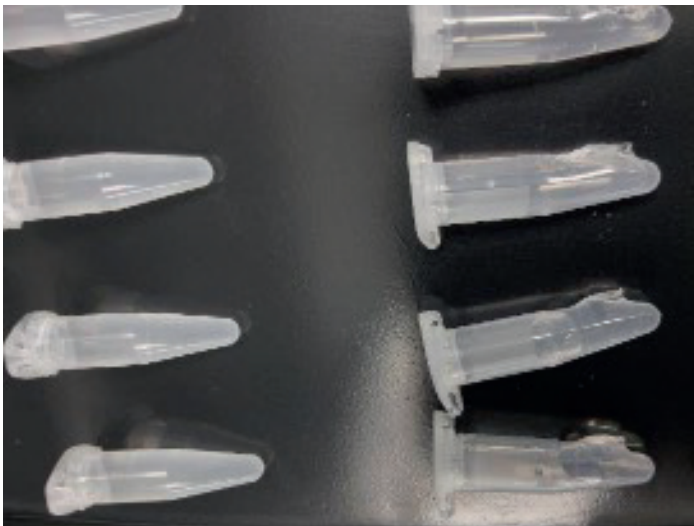
Figure 6: Comparison of Eppendorf 1.5 mL microtubes (left) with 1.5 mL biobased tubes of third-party supplier (right) after centrifugation at 22,000x g at up to +40°C
