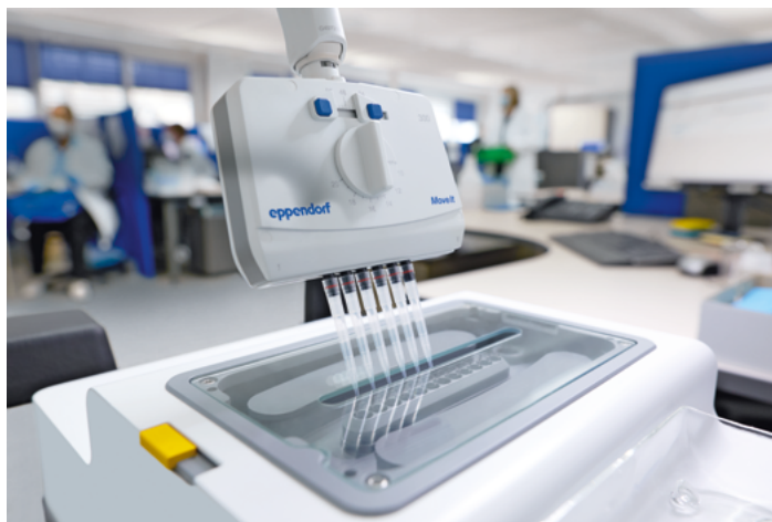
Figure 6: Gravimetric check of an Eppendorf multi-channel pipette with a multi-channel balance
