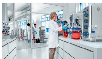
Cell Culture Scale-Up Using Stirred-Tank Single-Use Bioreactors
