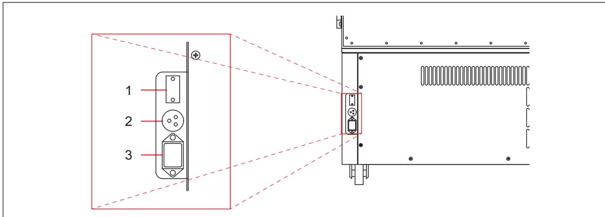
Fig. 6-3: Upright freezers alarm monitoring socket
