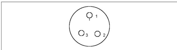
Fig. 6-6: Remote alarm socket - chest freezer
