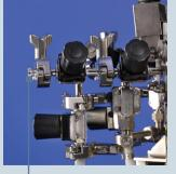
Resterilizable addition valve array: Each vessel can accommodate up to four addition ports for vessel additions (one addition port shown)
