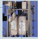
Optional glycol heat exchanger enables rapid cool-down; closedloop, eco-friendly design reduces need for single-pass cooling water through the system
