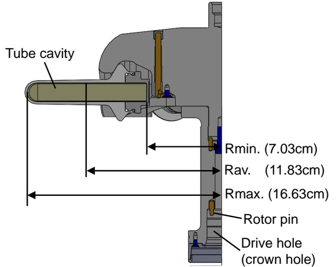
Fig.7-2. Cross-sectional view of P28S2 bucket
