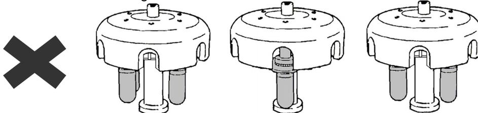
Tighten the cap to the bucket securely. Set the bucket to the rotor securely.
