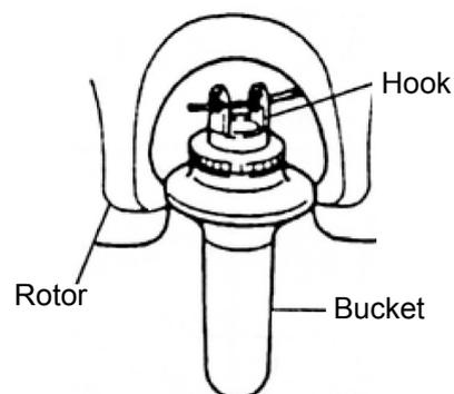
Hang the hook of the bucket on the pin of the rotor.
