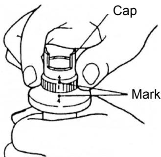
Tighten the numbered cap to the same numbered bucket to match each mark of the bucket and the cap.
