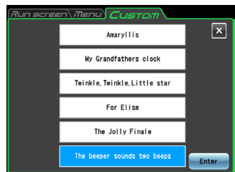
Fig. 3-4-5 (2) Stop signal setting screen
