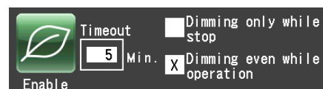
Fig. 3-4-5 (4b) Dialog box that appears when dimming backlight mode is enabled
