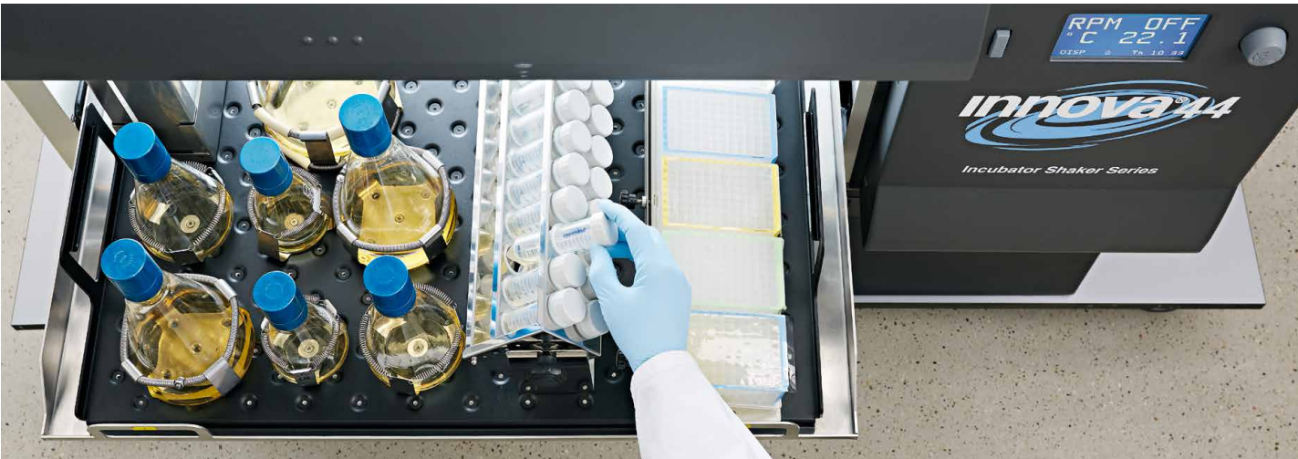
Slide-out platform mechanism — provides easy and effortless access to flasks located in the front and back of the shaker/incubator.
