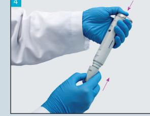
> Fit the ejector sleeve.
