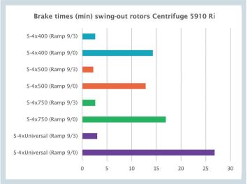
**Figure 5:** Brake times determined for the new Eppendorf Multipurpose Centrifuge 5910 Ri, used in combination with different swing-out rotors at ramp settings of either 9/0 or 9/3, respectively (rotors were fully loaded; the brake times decrease with decreasing load).
