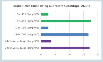
**Figure 4:** Brake times determined for the new Eppendorf Multipurpose Centrifuge 5920 R, used in combination with different swing-out rotors at ramp settings of either 9/0 or 9/3, respectively (rotors were fully loaded; the brake times decrease with decreasing load).
