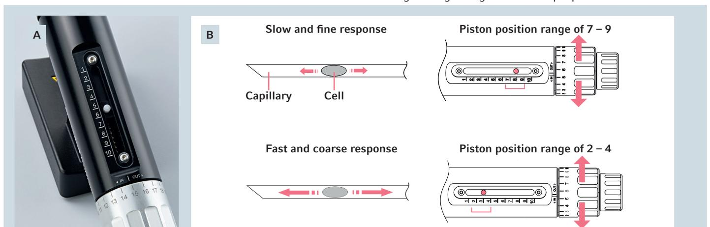
**Figure 1:** Adjustment of the responsiveness in pressure control of the CellTram 4r Air.
