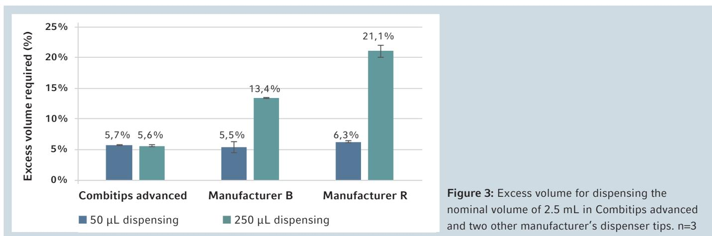
**Figure 3:** Excess volume for dispensing the nominal volume of 2.5 mL in Combitips advanced and two other manufacturer’s dispenser tips. n=3
