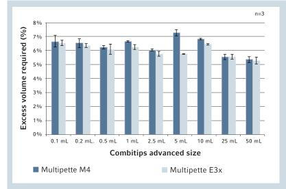
**Figure 2:** Excess volume required for complete filling of Combitips advanced dispenser tips using Multipette M4 or Multipette E3x ranges between 5.3 and 6.7%.
