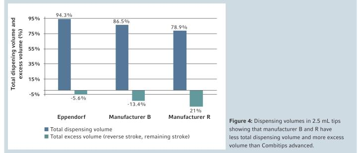
Figure 4 illustrates the percentage distribution of the filling volumes for 2.5 mL tips using 250  $\mu$ L dispensing steps. For 5 mL tips, the same relationship was determined. A significant amount of liquid needed as reverse and remaining stroke, volume in both competitor tips was visible. If the liquid was not re-dispensed into the source vessel it was wasted. This
