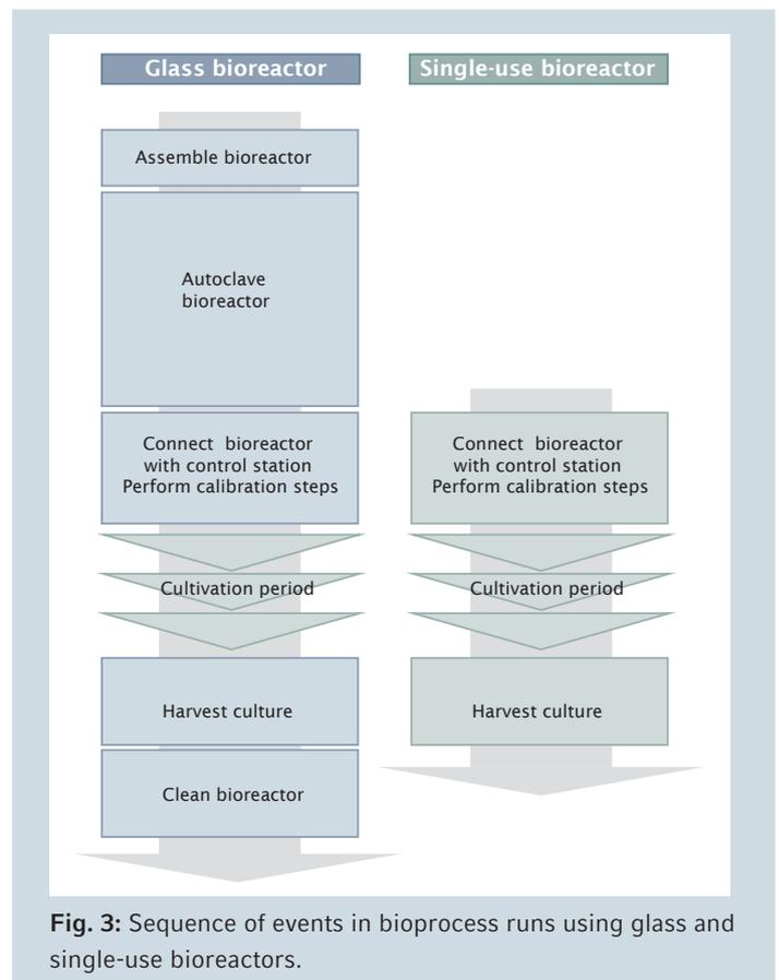
**Fig. 3:** Sequence of events in bioprocess runs using glass and single-use bioreactors.
