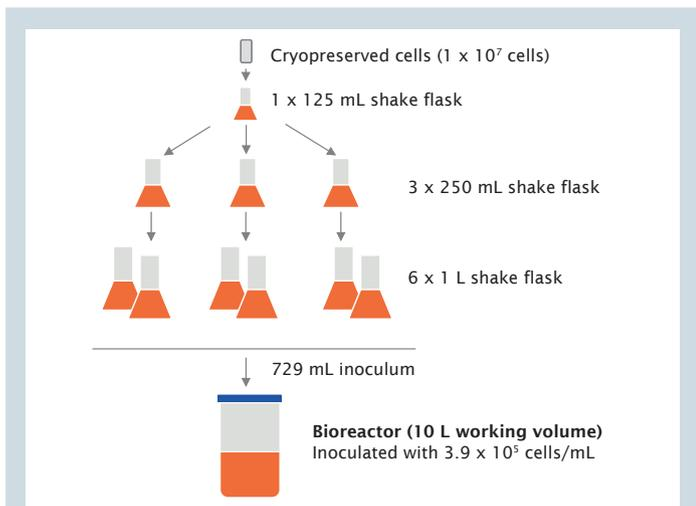
**Fig. 2:** Inoculum preparation for the bioprocess run.
