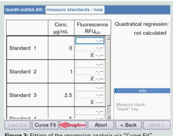
**Figure 3:** Fitting of the regression analysis via "Curve Fit" (red arrow).
