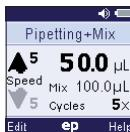
In addition, the display shows the mixing volume (*Mix*) and the number of mixing cycles (*Cycles*).
