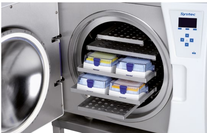
Figure 7: Autoclaving of lab consumables in a Systec autoclave (picture kindly provided by Systec)
