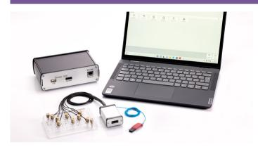
The performance of PCR cyclers depends heavily on temperature accuracy. However, Peltier elements can change accuracy over time! A regular PCR block temperature veri-fication increases reproducibility of PCR results.
