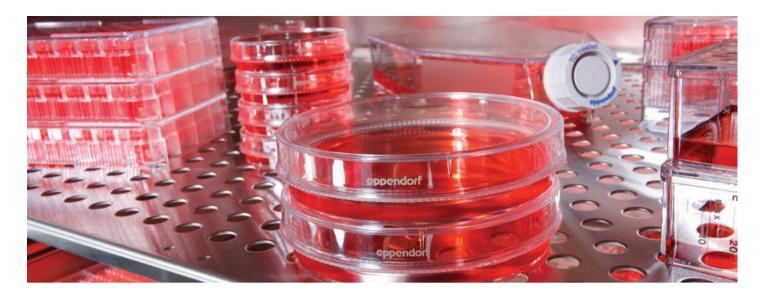
Vibration and turbulence protection by fanless design Have you ever experienced variations between cells grown in vessels on different shelves, especially between the top shelf and others? These differences can be caused by air turbulences that disrupt the protective micro-atmosphere above the medium. Air turbulence can be generated by fans used to circulate the atmosphere inside of standard
