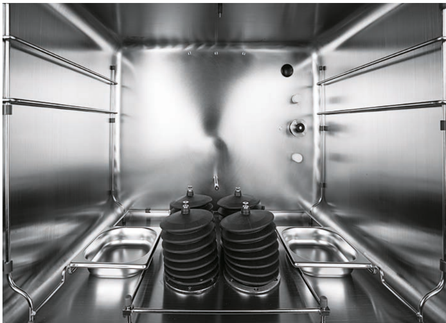
The seamless, deep-drawn chamber of the New Brunswick S41i with removable water trays. The high temperature-resistant rubber bellows protect the connection of the shaker drive with the platform (not installed here).
