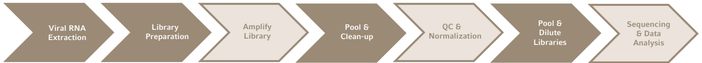
Figure 1: Automated workflow for the Illumina® COVIDseq™ Test on the epMotion® 5075t NGS Solution. Steps shown in brown can be automated on the epMotion® liquid handler.
