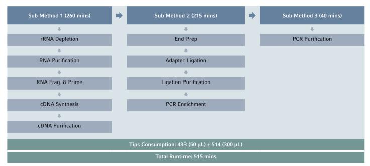
**Figure 3:** Workflow of the NEBNext<sup>®</sup> Ultra<sup>™</sup> II Directional RNA Library Prep with rRNA Depletion protocol on ep*Motion*<sup>®</sup>. The steps are grouped into ep*Motion*<sup>®</sup> sub-methods. The methods are optimized for up to 24 samples. ep*Motion*<sup>®</sup> runtime and tip consumption estimate is for 24 samples.
