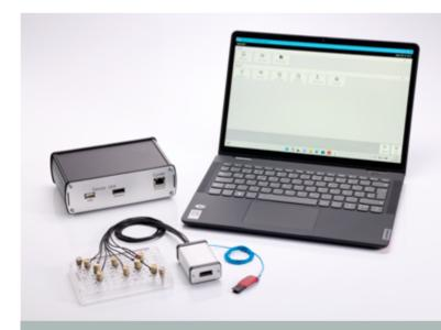
Temperature verification with a multi-probe system allows fast and reliable assessment of the cycler's performance. The generated certificates can support instrument qualification for your quality management system.
