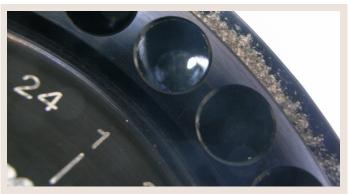
Figure 1: Localized corrosion in bore hole
