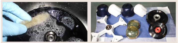
**Figure 4:** Clean rotor and rotor bores with plastic scrub pad and/or stiff test-tube brush in case of stubborn stain. Then rinse with water and dry.
