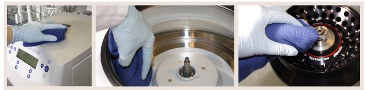
Figure 2: Wipe outside of centrifuge and clean rotor chamber and rotor with moist cloth and neutral detergents.
