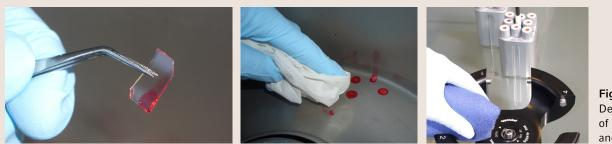
**Figure 3:** Decontamination of centrifuge, rotor and rotor buckets.
