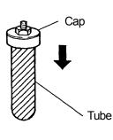
(2) Tighten the nut of the cap with the box wrench.
