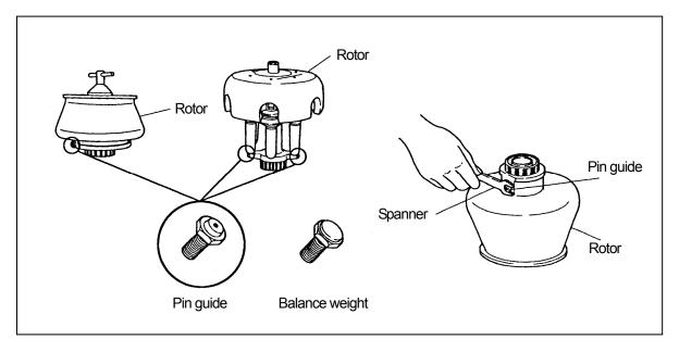
Fig.4-4 Pin guide attachment positions and how to attach
