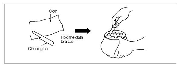
Fig.4-2 How to the use a cleaning bar
