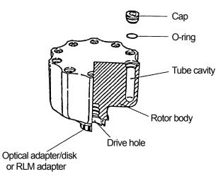
Fig. 1-4 Names of parts of vertical rotor
