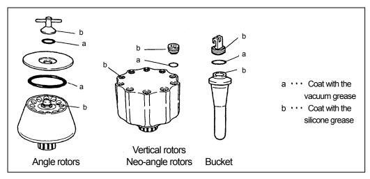
Fig.4-1 Coating the grease
