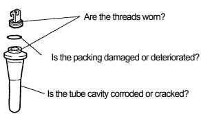
CAUTION : Check the packing (O-ring) every time. Replace it with new one if deterioration (crack, deformation, etc.) is observed. Otherwise, samples might be damaged due to poor rotor seal or the centrifuge or the rotor might be damaged during operation.
