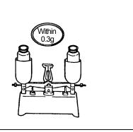
NOTE: Although you balanced the bottles within the approximate allowable imbalance (5mm), alarm message "IMBALANCE" might appear. Balance bottles more accurately again if the alarm message "IMBALANCE" appears (see the rotor instruction manual).
