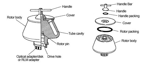
Fig. 1-1 Names of parts of angle rotor
