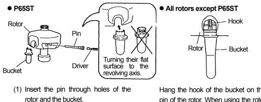
Hang the hook of the bucket on the pin of the rotor. When using the rotor which has two hooks, make sure that both hooks hang on the pin.
