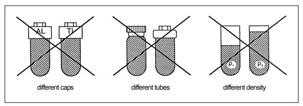
Fig. 2-7 Correct balancing
