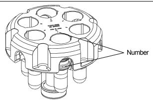
Match numbered buckets with number of rotor and set the buckets to the rotor.
