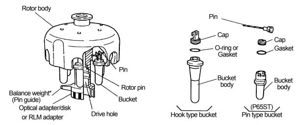
Swing rotors (hook type buckets and pin type buckets) other than the P32ST rotor and the P32ST2 rotor
