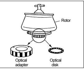
Fig. 1-5 Optical adapter/disk
