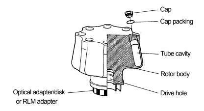
Fig. 1-2 Names of parts of Neo-angle Rotor
