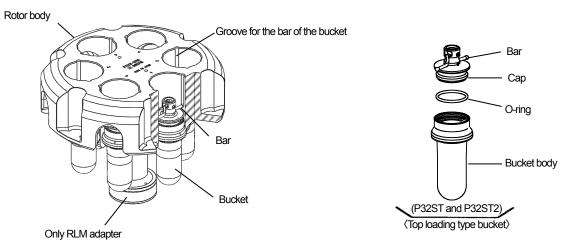
Fig. 1-3 Names of parts of swing rotor
