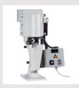
Figure 1: The CEPA LE is a benchtop laboratory centrifuge, featuring variable speed contol as standard and a wide array of optional bowls for research, scaleup experiments, and small volume production. The LE is typically used with 2 to 15 liter cultures. Maximum throughput is 30 liters/hour.
