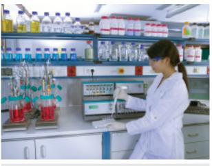
Parallel benchtop bioreactor system for cell culture
