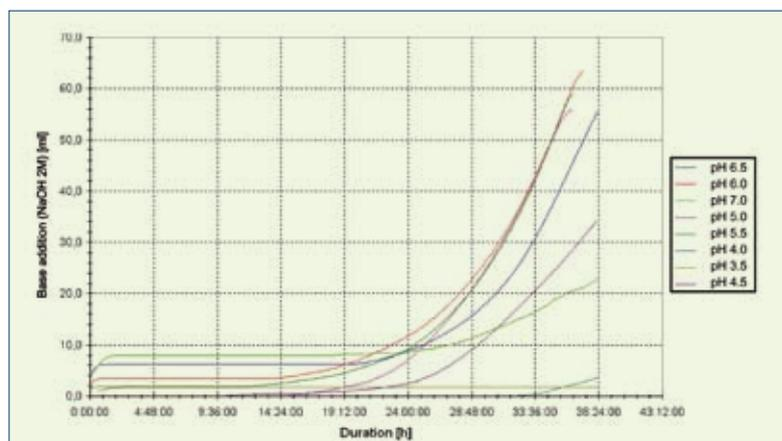
Figure 3. DASGIP parallel bioreactor systems are designed to meet the specific needs of process optimisation. Scientists can compare the efficiency of the key parameters, here different pH values are plotted from eight reactors in parallel.
