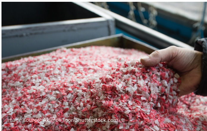
Mechanically ground plastic
