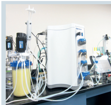
Fig. 8: High-density E. coli culture in the BioBLU 3f Single-Use Vessel. Fed batch fermentation process 11 hours post inoculation.
