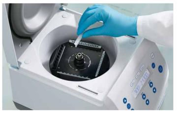
Centrifuge 5420 offers two rotor options: A 24-place standard rotor for up to 24  $\times$  1.5 or 2.0 mL tubes and a PCR-tube rotor for 4  $\times$  PCR strip or 32  $\times$  PCR tubes (0.2 mL).
