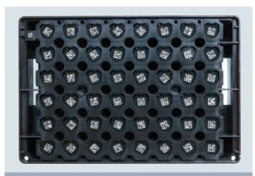
With the Eppendorf RackScan and software, you can scan more than one vial in parallel and transfer the sample data to your sample management software, e.g. eLABInventory or external databases
